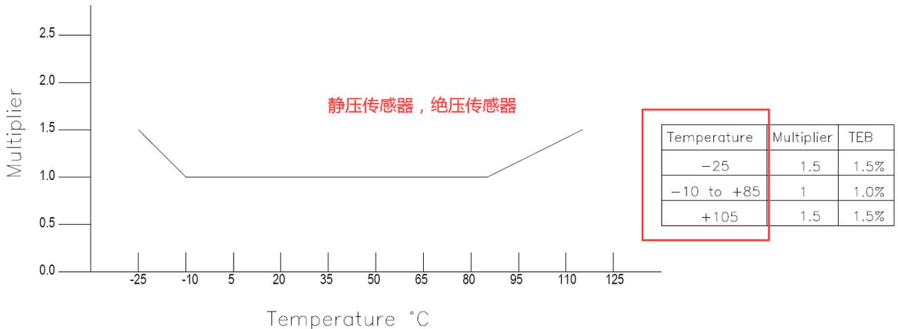
NOTE: The Multiplier is a linear response from -10°C to -25°C and from 85°C to 105°C.
