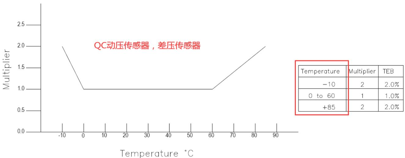
NOTE: The Multiplier is a linear response from 0°C to -10°C and from 60°C to 85°C.
